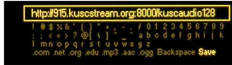
The entry method is self-explanatory, but you may find it necessary to search the station’s Website to find the right streaming address, often including a port number as shown in this example.
