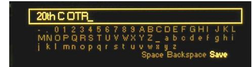
The list may be re-ordered through a slightly convoluted process. You may move any existing preset to the top of the list by making it the ‘Now Playing’ station and renaming it with the same name. You’ll then have two identical listings, and the duplicate underneath may be deleted. Repeat as necessary to get the list sorted to your satisfaction.
