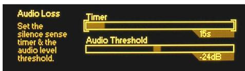
The Timer slider sets the number of seconds between the onset of ‘dead air’ and the alarm. How this is set may depend on the stream format. A classical music or an oral interpretation stream might call for a setting of 30 seconds or more to allow for the soft passages or long pauses inherent in these formats. A high-energy music outlet, on the other hand, could be safe with a 10-second setting.
