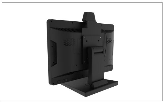
Aline the 4 screws holes at the back of TAURI to FIX-028 Table Stand screw positions, and place screws to fixate it.
