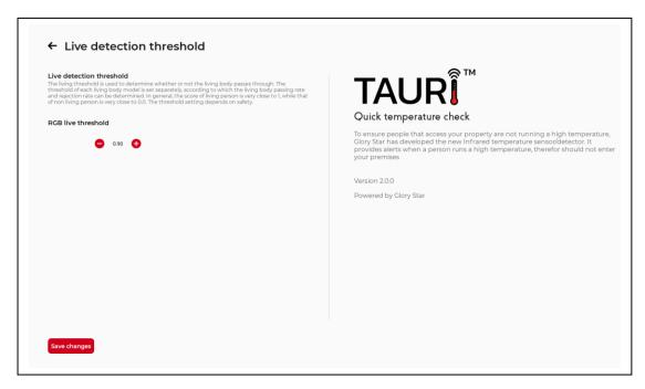
**8.9 Live detection threshold:** Adjust the value to check whether the target object is a living object or not.
