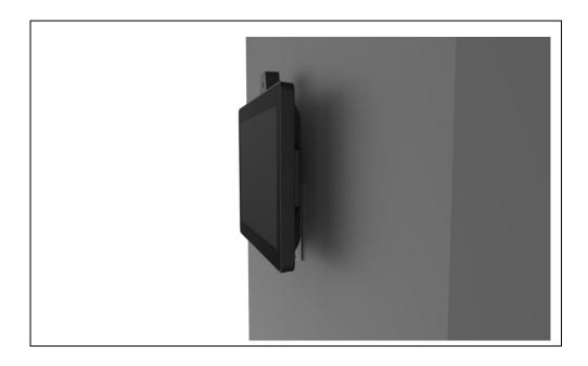
Slide TAURI with the wall mount on to the mount on wall using the hinges at the side of the wall mount.
