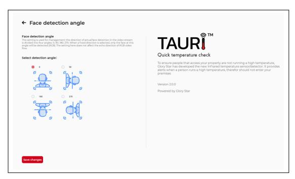
**8.5 Face detection angle:** Adjust the detect angle of the person's face (for the device put in portrait or landscape position).
