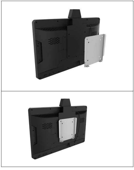
Install the wall mount to the back of the device and put screws on the 4 holes of the mount aligning to the TAURI's back mount holes.
