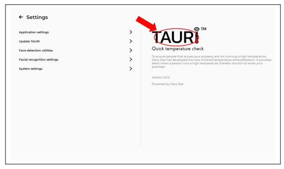
4.Thermographic calibration is hidden from the manual for security. **Tap the**"TAURI logo" on main setting page 5 times to start calibration.
