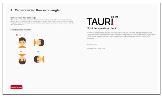
**8.6 Camera video flow echo angle:** Adjust the image direction of the output video stream.
