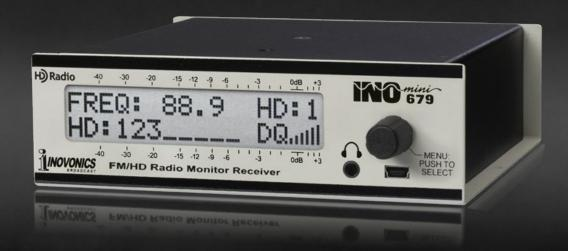
The INOmini 679 is Inovonics' third-generation, small form-factor FM and FM-band HD Radio broadcast monitor receiver, demodulating both analog FM and digital HD1-HD8 radio channels for confidence monitoring. You get a high-quality audio feed for rebroadcast or program distribution throughout the broadcast facility with adjustable analog and AES digital audio outputs. FM RBDS and HD Radio PAD data may be called-up for display on the front-panel LCD screen.
