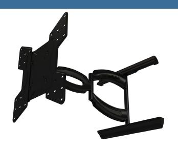
Articulating mount for 32" to 75" displays. Multiple joint arm holds display 3.5" from wall when retracted and 27" when fully extended. Smooth tilt adjustments of  $+15^{\circ}$  (forward) and  $-5^{\circ}$  (back) with a locking knob and 3° side-to-side roll facilitates a variety of viewing angles and perfect positioning. Integrated cable management for clean look.
