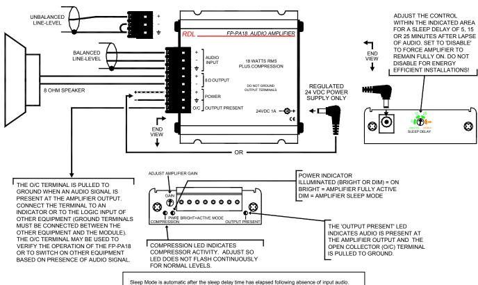
Sleep Mode may be activated manually by repowering the module with input audio absent.
