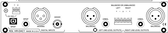
Connect one digital audio source to the appropriate input jack:
