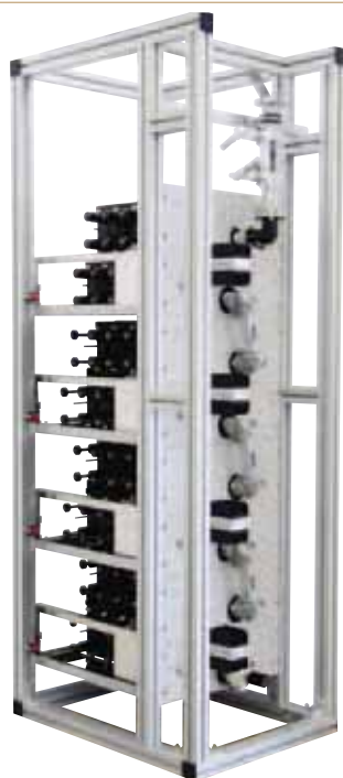
BN 57 52 72 5-way combiner with integrated DTV mask filters
