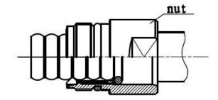
3. Set the nut onto the outer conductor of the cable as shown.
