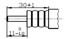
1. Trim the end of cable straight, and then strip the sheath as shown with a knife. Be careful not to nick the outer conductor.
