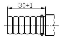
2. Set the O-Ring into the trough as shown.
