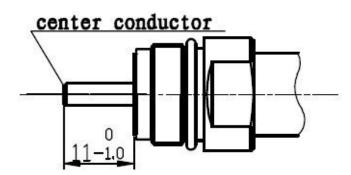
5. Cut through the foam dielectric against the edge of the nut, and then completely remove the foam dielectric from the exposed section of the center conductor. Chamfer the end of the conductor with a hand file as shown.
