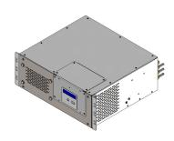
DryLine® Dehydrator, Low-pressure membrane, 19 in rack mountable, Wall mountable, Cut-in at 2.0 psi, Cut-out at 5.0 psi, with discrete and summary alarms, 115/230 Vac, 50/60 Hz
